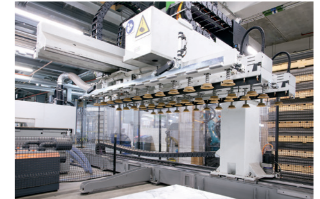
The Synchro operates along a track, loading and unloading two panels at a time.
